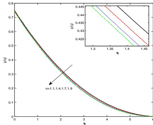
Fig.4 Effect of power law index  $n$  on  $\phi(\eta)$
