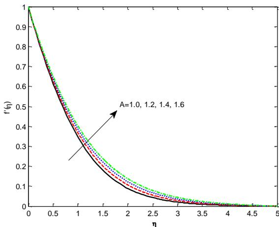
Fig.22. Effect of material parameter  $A$  on  $f'(\eta)$
