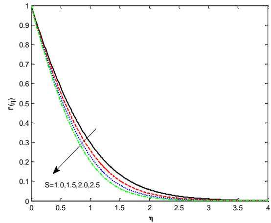
Fig.6. Effect of stretching parameter  $s$  on  $f'(\eta)$
