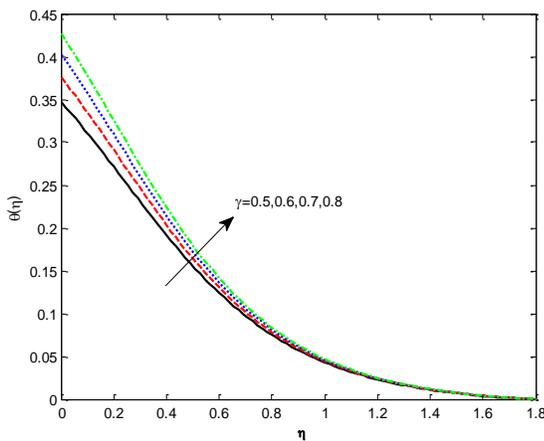
Fig.10. Effect of Biot number  $\gamma$  on  $\theta(\eta)$
